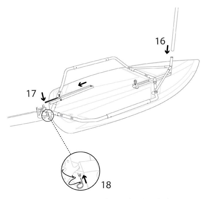
Before going sailing, make sure the safety pin is inserted in the hole of the rudder pintle (upper).
